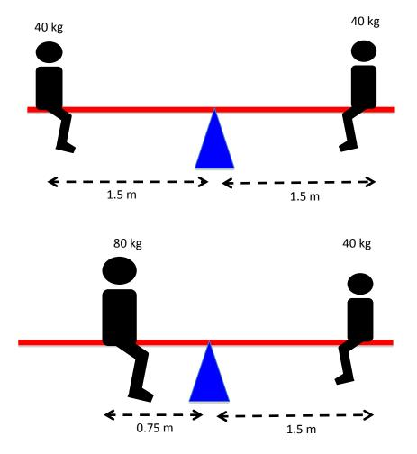
This same lever principle also allows us to lift very heavy loads with little effort provided that the lever we use is long enough and the fulcrum is placed close to the load.
